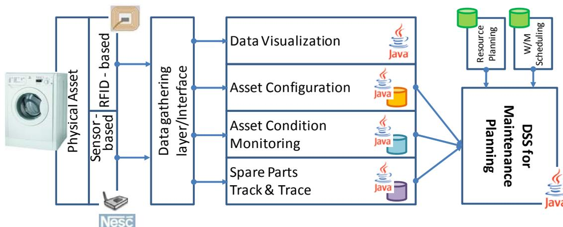
Figure 1. The architecture of the demonstrator
