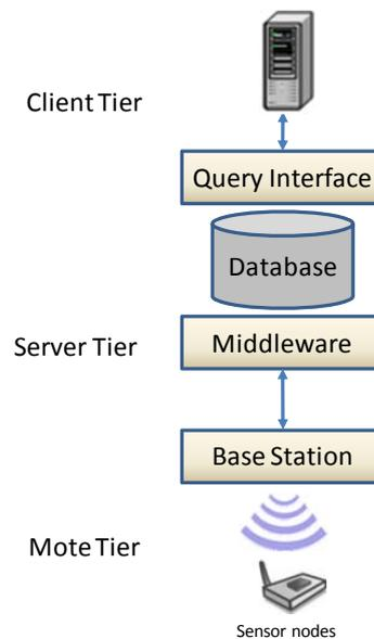
Figure 5. System architecture for condition monitoring [7]
