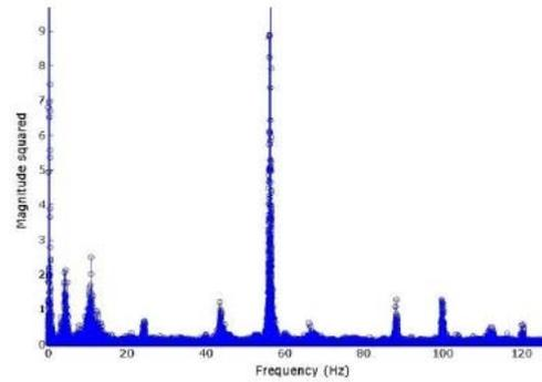
Figure 6. Vibration spectrum of drum from acceleration data obtained in a single washing machine cycle
