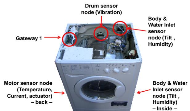
Figure 3. Deployment of sensors on the washing machine
